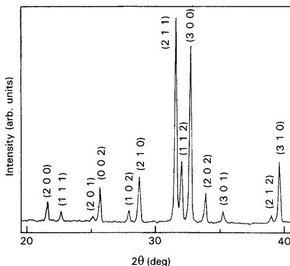
Figure 2 An XRD ( $\text{CuK}\alpha$ ) pattern of HAp whiskers showing their high crystallinity and the non-existence of phases other than hydroxyapatite. The numbers in parenthesis indicate the plane indices, based on the hexagonal space group.
