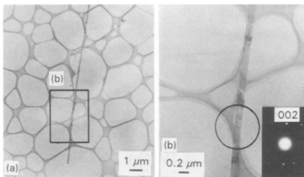
Figure 4 Transmission electron micrographs of: (a) a HAp whisker; and (b) an enlargement of (a) and a selected-area diffraction pattern from the area indicated by the circle, showing that the HAp whisker is a single crystal elongated along the *c*-axis.
