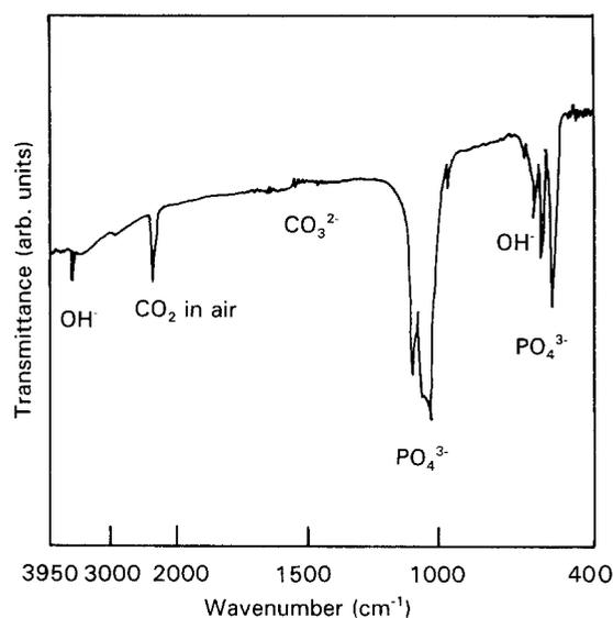
Figure 3 Infrared spectra of HAp whiskers indicating some internal vibrational peaks characteristic of hydroxyapatite.
