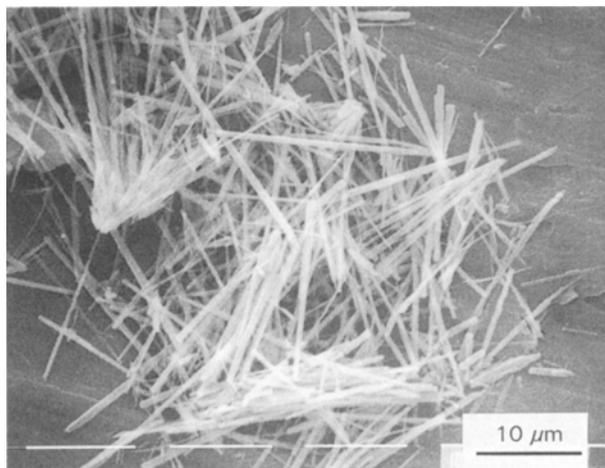
Figure 1 Scanning electron micrograph of HAp whiskers prepared by the hydrothermal treatment of beta-TCP with citric acid at 200 °C at 2 MPa for 1 h.
